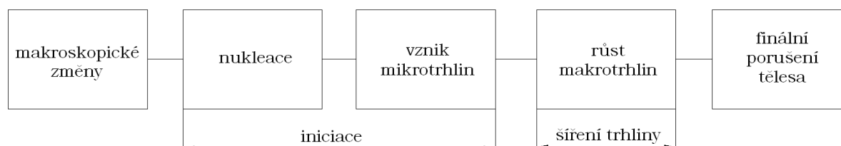
Fig 6.2 Chronology of individual stages of the fatigue process in an object without technological defects.
