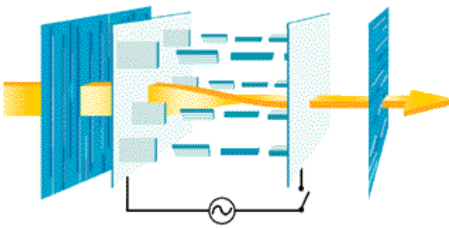
Fig. 7.8 a) Idle state – the light is allowed to pass
