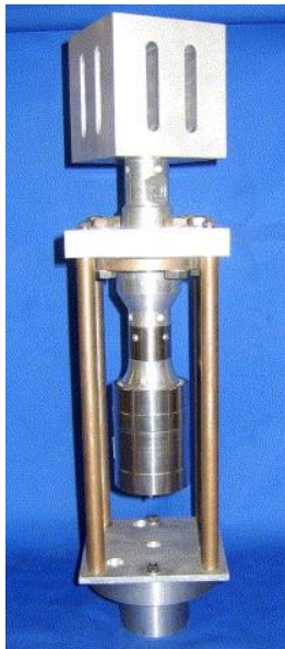
Fig. 1. Double-slotted block horn and ultrasonic transducer with attached mounting structure for ultrasonic compression tests.
