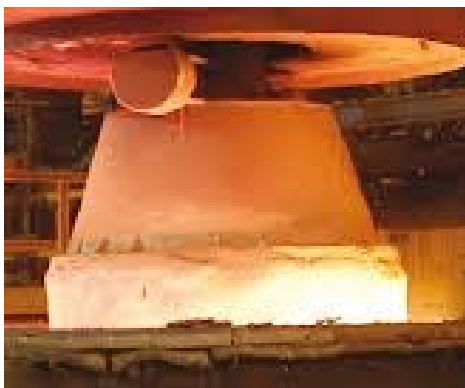
a) snorkel of CAS-OB ladle furnace in operation
