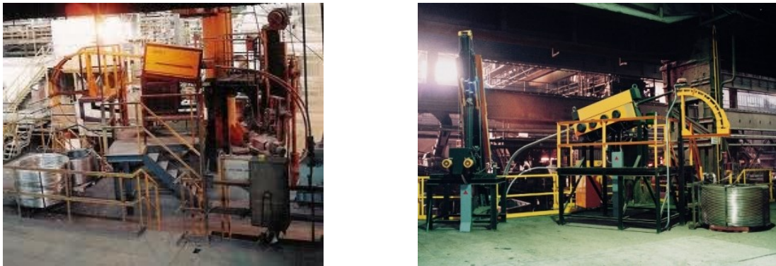
Fig. 30 Example of equipment for inputting Al wire and cored wires
