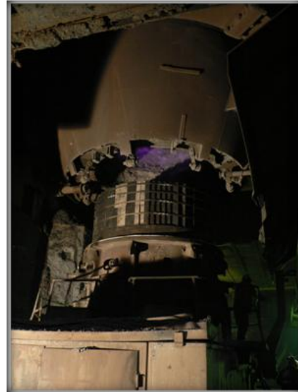
Fig. 15 An exchangeable bottom and its installation into a converter
