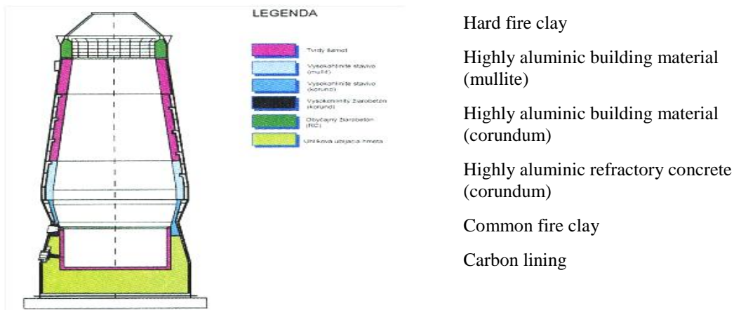
Fig 11 A detailed diagram of a classically brick-lined blast furnace
