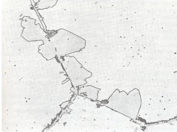
*Fig. 6.25 Massive  $\alpha$  phase grains at grain boundaries of  $\beta$  in the alloy Cu – 38 at. % Zn hardened at the temperature of 850°C using ice brine at 0°C. Dark particles along the grain interfaces represent precipitates that developed by means of the nucleation and growth mechanism (precipitation) at a high temperature.*
