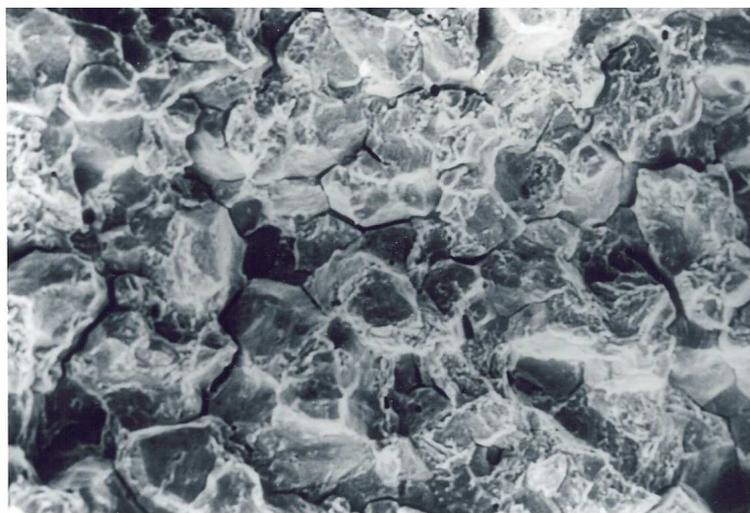
Fig. 6.5 Morphology of the fracture surface produced by the stable crack growth in high strength steel 38MnSiCr2Ni2Mo due to stress corrosion cracking in 70°C hot water
