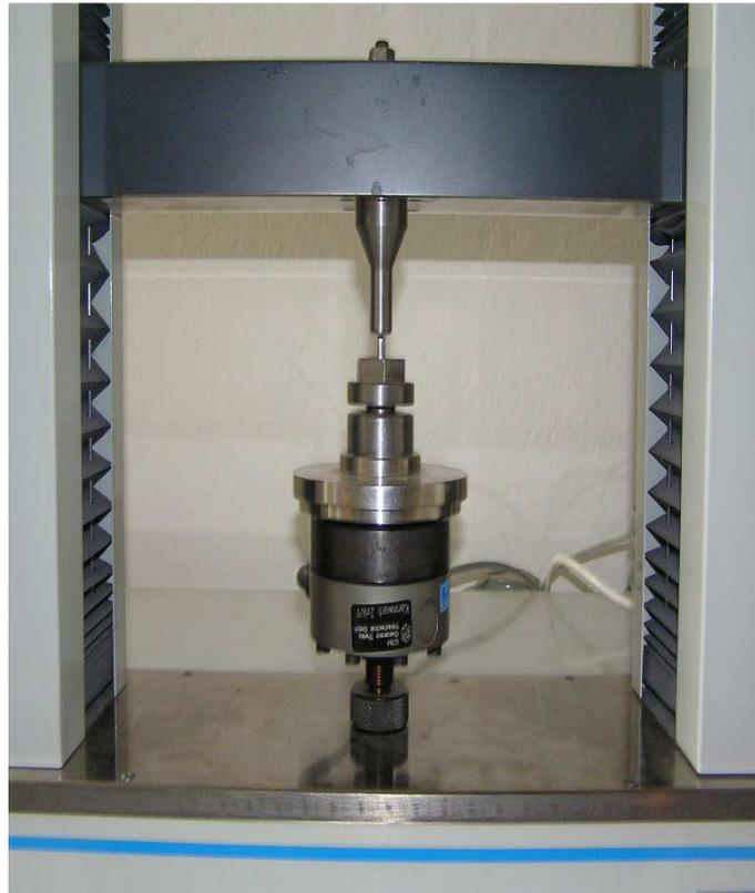
Fig. 8.4 Laying of test jig in the frame of the testing device
