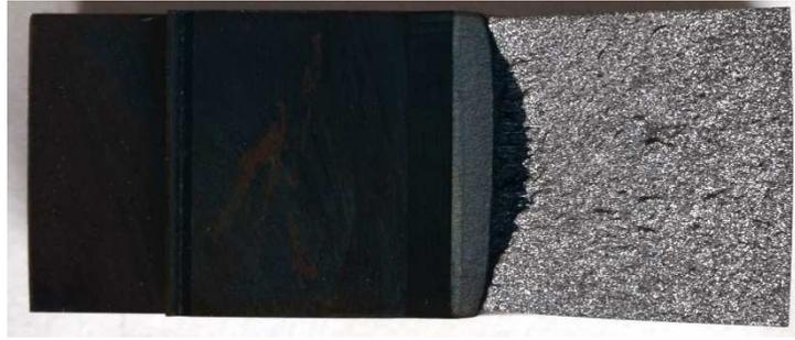
Fig. 4.28 Stable crack growth highlighted by staining specimen after its relieving in an oven at 300°C and after being broken apart in liquid nitrogen
