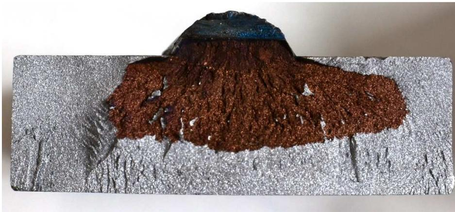
Fig. 4.8 Specimen intact during the drop-weight test. Fracture in the base material did not extend to either one or both edges of the specimen.
