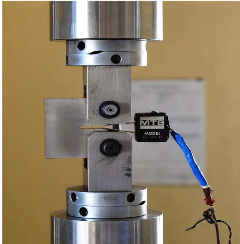
Fig. 4.21 Experimental test of fracture toughness at room temperature using the compact tension specimen
