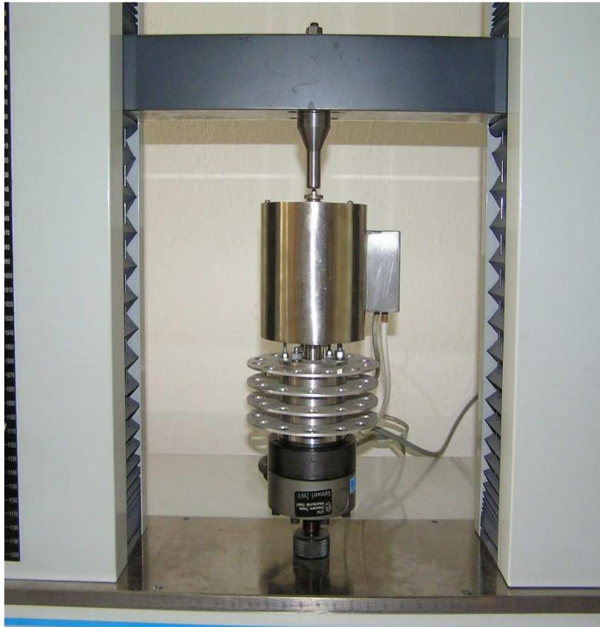
Fig. 8.15 Test equipment for penetration tests at elevated temperatures (up to 400°C)
