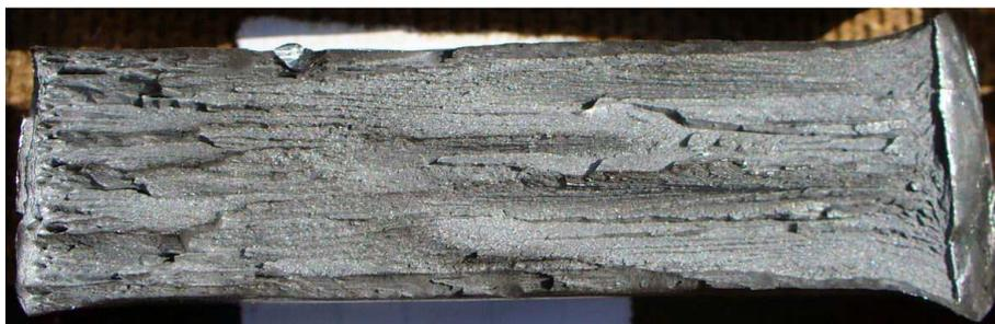
Fig. 4.13 Test temperature  $-60^{\circ}\text{C}$ , proportion of ductile fracture 10%
