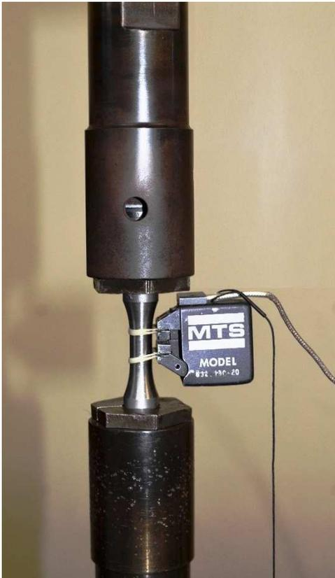
Fig. 3.8 Smooth cylindrical test body with a longitudinal strain sensor
