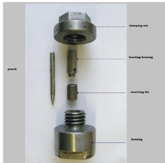
Fig. 8.3 Test jig for ball “Bulge” test at room temperature
