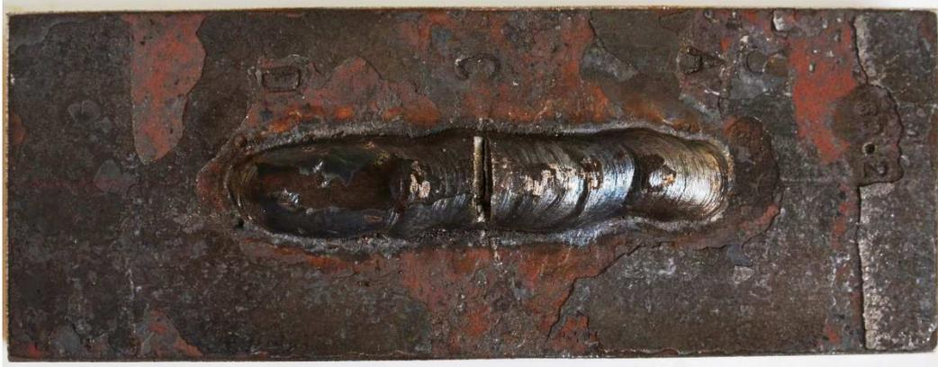
Fig. 4.7 Specimen with dimensions 16 x 50 x 130 mm used for DWT
