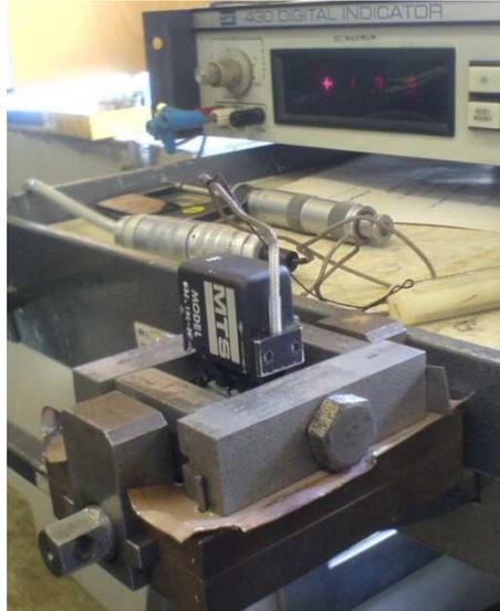
Fig. 7.16 The procedure of loading specimens in a test frame
