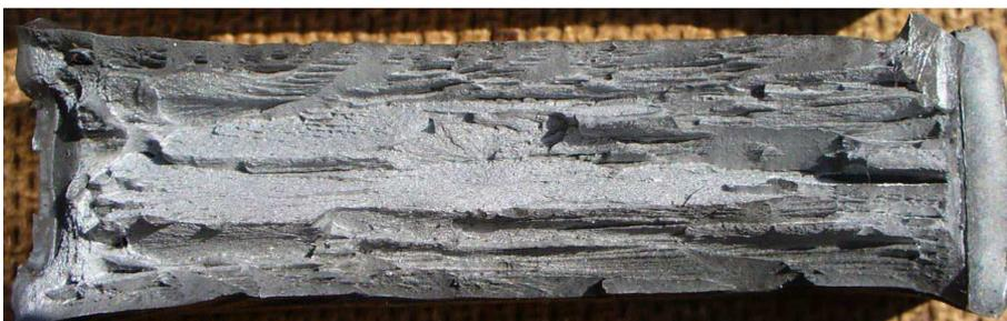
Fig. 4.12 Test temperature  $-40^{\circ}\text{C}$ , proportion of ductile fracture 45%
