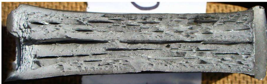
Fig. 4.11 Room temperature, proportion of ductile fracture 100%
