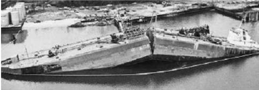
Fig. 2.1 Sudden unstable failure of a welded Liberty-class ship
