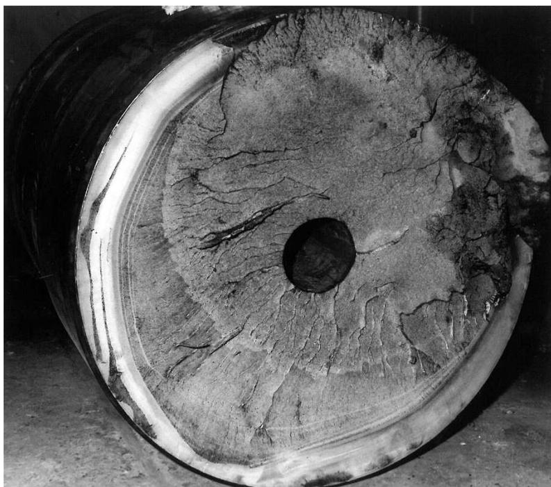
Fig. 3.2 Fatigue fracture of the shaft of the wheel of giant machine K 10000
