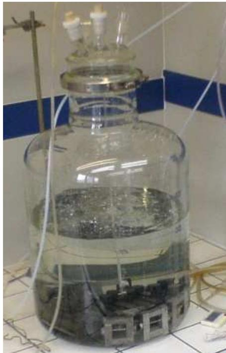
Fig. 7.17 Exposure of specimens loaded in test frames according to ASTM Standard G 49-85
