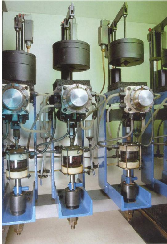
Fig. 7.12 Dead Weight Device in Arcelor Mittal Ostrava
