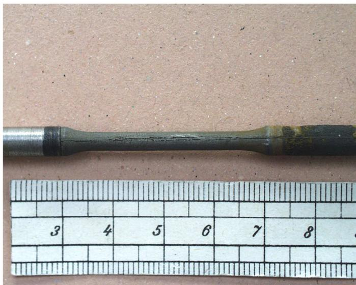
Fig. 7.11 Longitudinal cracks on the specific part of the test bar after SSC test – X70 grade steel
