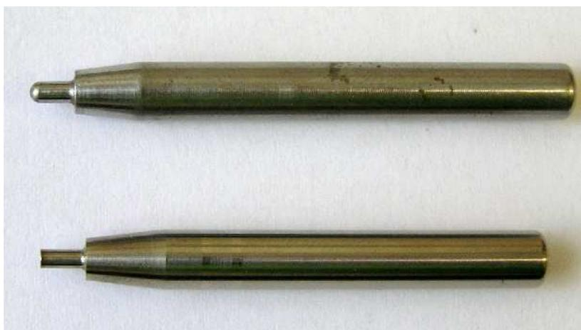
Fig. 8.2 Shape of punch used for ball and shear tests
