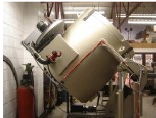
Fig. 11.3 Crucible induction furnace of Stinchcombe Furnaces Group, s.r.o.
