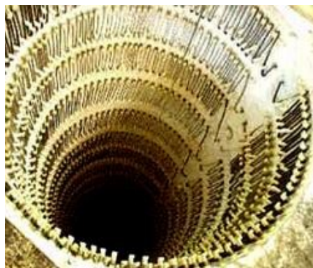
Fig. 11.5 Soaking furnace with resistance heating
