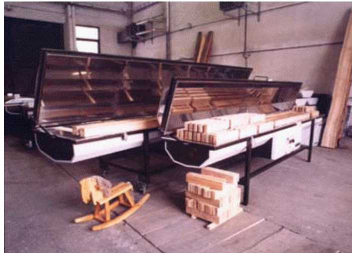
Fig. 11.6 Device using dielectric heating for drying wood
