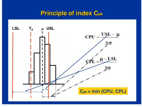
Fig. 3.10 Principle of index Cpk
