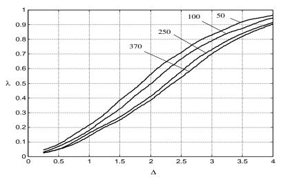
Fig. 8.3 Nomogram for optimal  $\lambda$  vs. shift  $\Delta$
