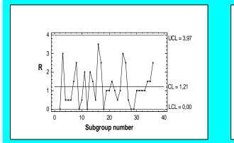
Fig. 12.1 Control chart for moving ranges
