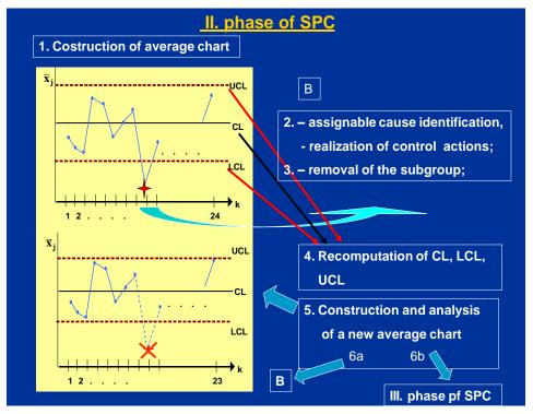
Fig. 3.7 II. phase of SPC – construction and analysis of control chart ( $\overline{X}$ )
