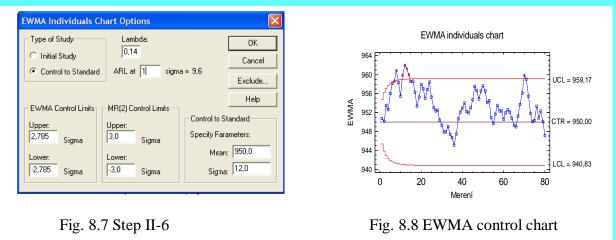
Based on Fig. 8.8 we can conclude that the analyzed process is not statistically stable (it is out of control).
