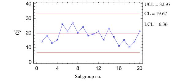
Fig. 6.11 Application of control chart (c) in IV. phase of SPC
