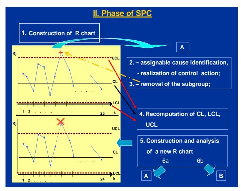
Fig. 3.6 II. phase of SPC – construction and analysis of control chart (R)
