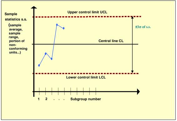
Fig. 3.1 Basic structure of control chart
