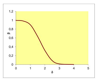
Fig. 5.1 Example of OC for an average control chart
