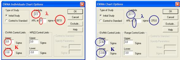
Fig. 8.2 Influence of changes of  $\lambda$  and upper and lower sigma for setting EWMA control limits K on the ARL value
