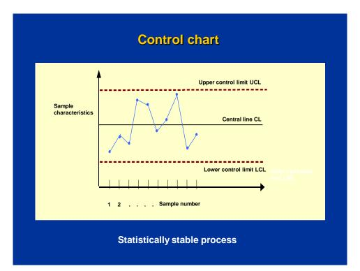
Fig. 1.5 Example of a control chart for statistically stable process
