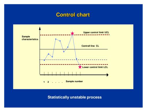
Fig. 1.6 Example of a control chart for statistically unstable process
