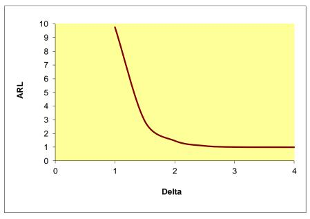
Fig. 5.2 Example of the ARL curve for an average control chart
