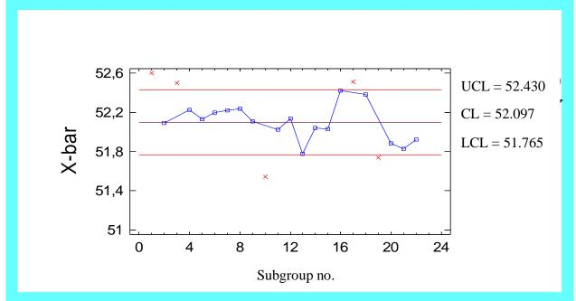
Fig. 6.16 Control chart  $\overline{\mathbf{x}}$  with recomputed CL, LCL a UCL
