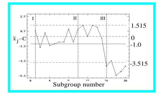
Fig. 7.9 Example of target control chart for averages
