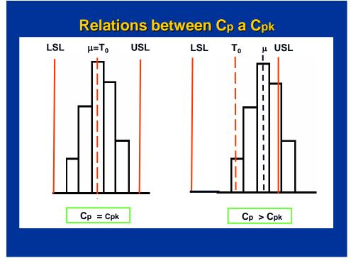
Fig. 3.12 Relations between indices  $C_p$  and  $C_{pk}$  (drift to USL)
