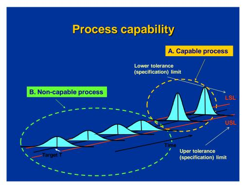
Fig. 1.7 Capable and non-capable process
