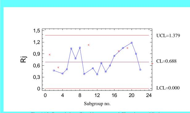
Fig. 6.15 Control chart (R) with recomputed CL and control limits
