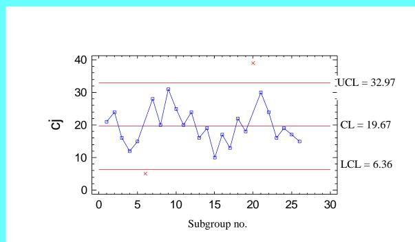
Fig. 6.10 Control chart (c) with recomputed control limits
