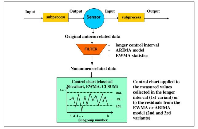
Fig. 7.7 Principle of the solution of the data autocorrelation: variants 1-3
