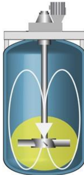
Fig. 3.5 Leaching tanks with agitators [5].
