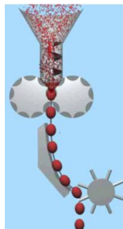
Fig. 1.8 Briquetting of fine-grained ores and concentrates.
