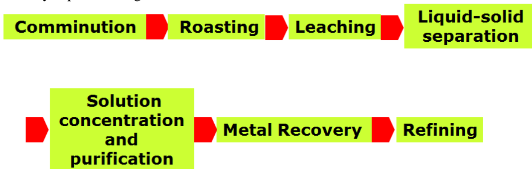
Fig. 3.1 Basic steps of hydrometallurgical metals production.
