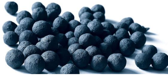
Fig. 1.9 Pellets from fine-grained ores and concentrates [9].
